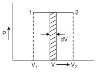
Work done in the expansion of a gas from volume  $V_1$  to  $V_2$  under constant pressure 'P' is equal to the area under P – V diagram.
